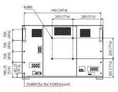
To install on avehicle, fix the unit using screw holes for the YOKE mount.
