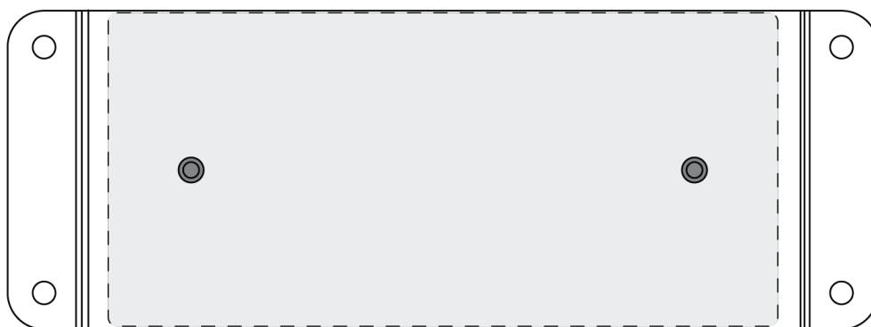
Align the holes as shown for securing a single device in the single-unit mounting tray
