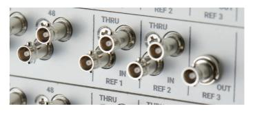
In remote setups, an .edge unit in a flypack can receive PTP timing via the network and provide tri-level sync to non-PTP capable devices. This removes the need for an external, on-location synchronous pulse generator (SPG).
