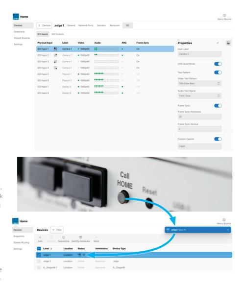
Conversely, operators can click a dedicated button in HOME to cause the ID indicator on a processing blade to flash, making it easy to troubleshoot cabling issues.
