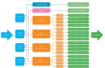
On the output side, 4 x 4 audio receivers each support 64 audio channels and can output 32 of them. Support for a combined 128 audio channels (4 x 32 ch.), as defined for the 12G/Quad-Link standard, is invaluable in production scenarios that involve parallel combinations of immersive, 5.1, stereo, and other audio formats.
