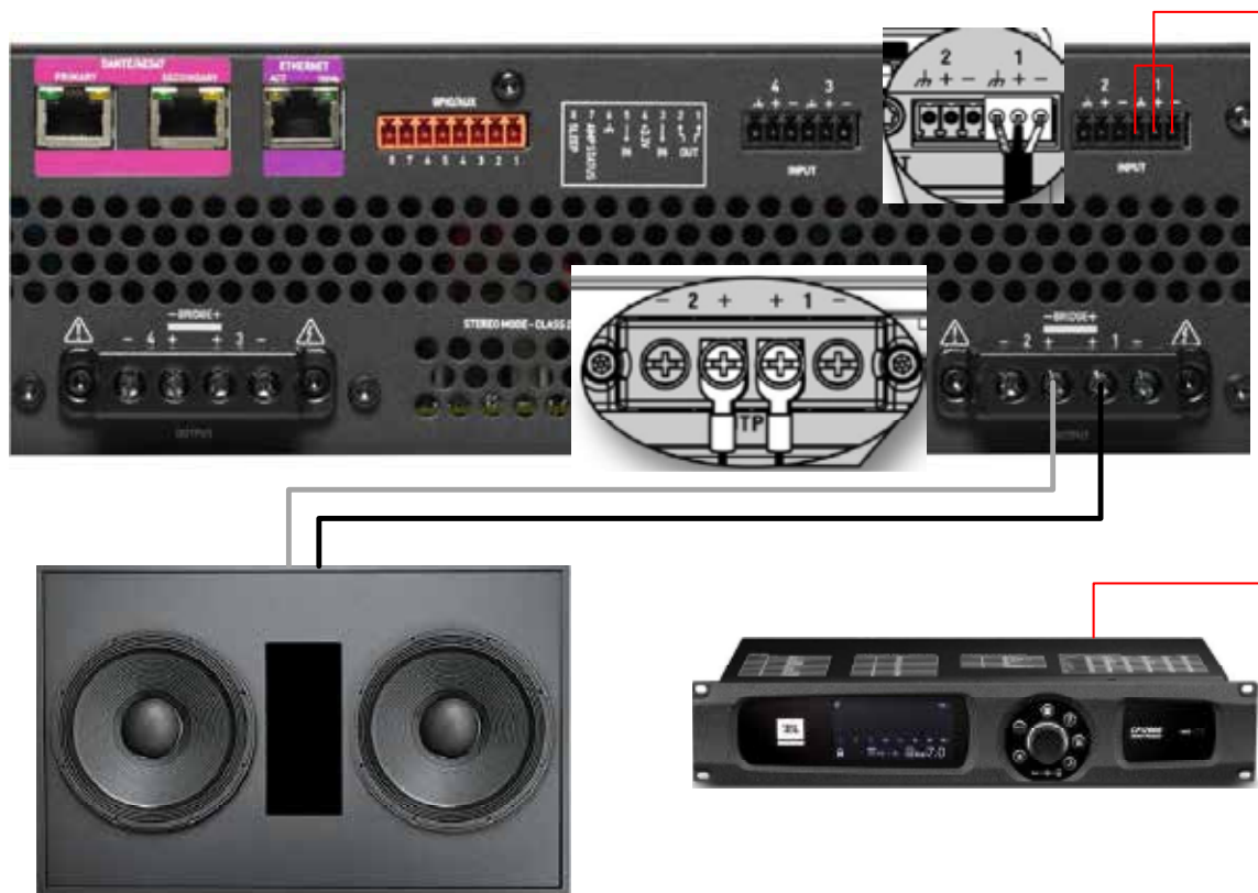
Figure 61: System wiring in Bridge Mono mode
