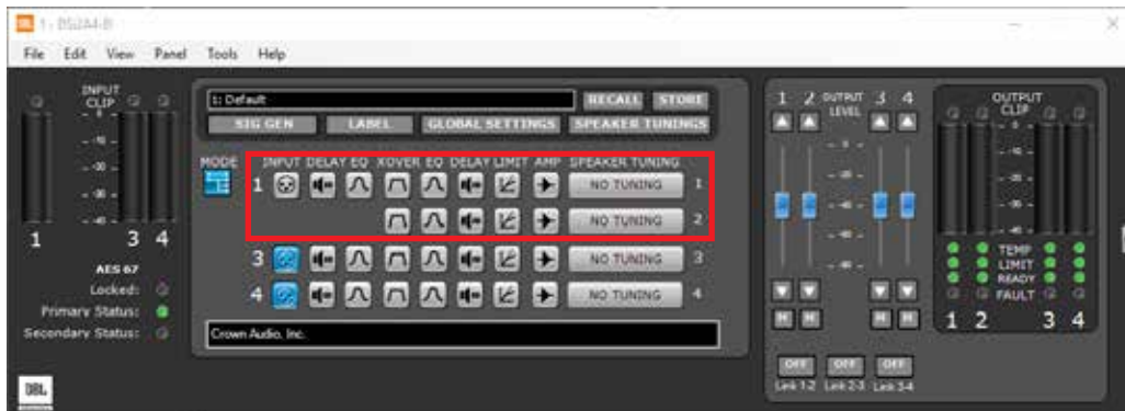
Figure 42: With the "Y 1+2" box checked, both output Ch.1 and Ch.2 are fed by input Ch.1 and input processing is organized accordingly
