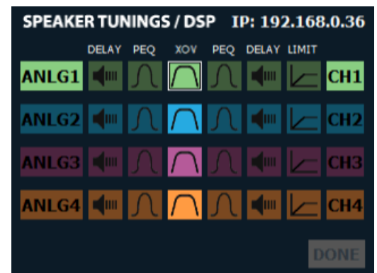
Figure 16: Speaker Tunings/DSP screen
