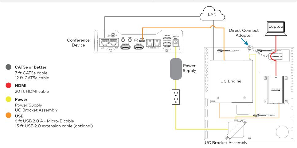
3. Connect the display and camera as shown below.
