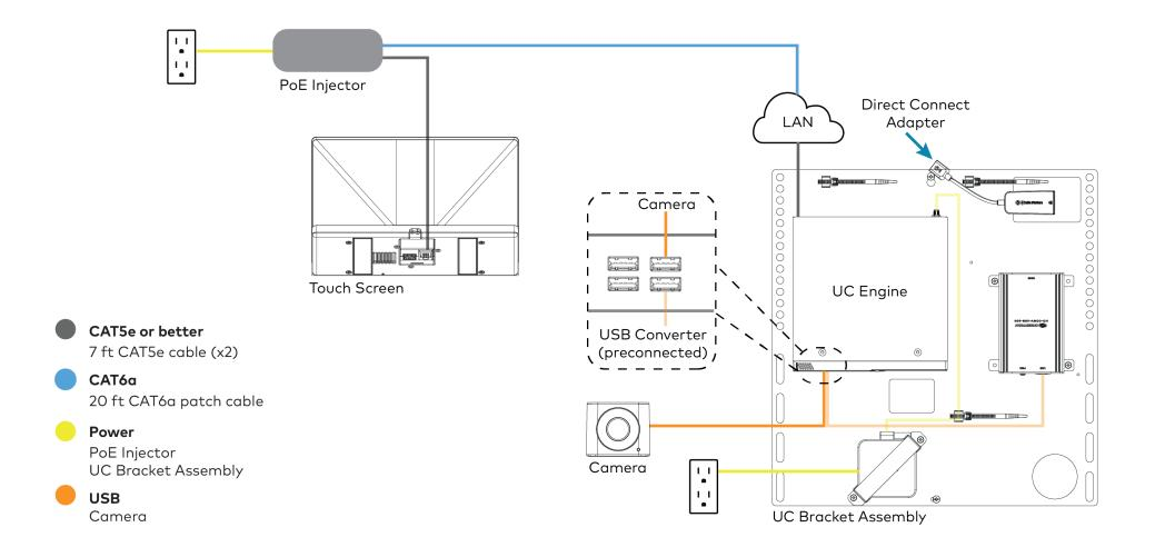
3. Make the remaining system connections as shown below.
