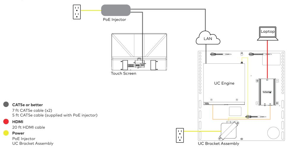
3. Make the remaining system connections as shown below.
