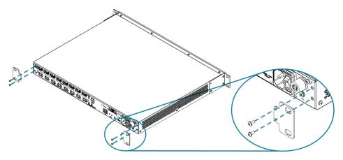
Then mount the device into the rack using four rack mounting screws (not included).
