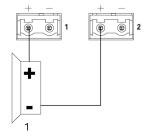
Speakers are bridged with the Crestron Avia™ Audio tool, which can be downloaded from <a href="www.crestron.com/software">www.crestron.com/software</a>. The possible bridging combinations are Output 1 & Output 2, Output 3 & Output 4, Output 5 & Output 6, and Output 7 & Output 8.
