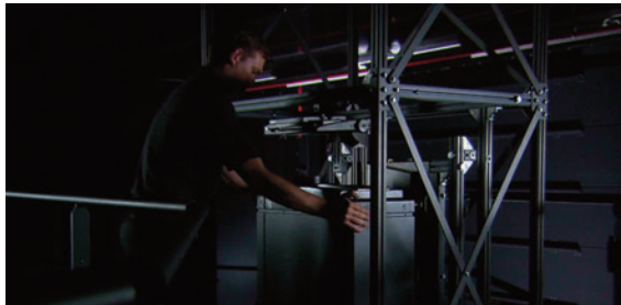
Projectors can be rolled in and out easily for quick part replacements.
